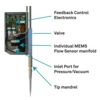
An inlet port provides aspiration/dispense pressure to the channel. A solenoid valve is coupled to a silicon MEMS flow sensor that controls the pipetted volume and allows precise tracking of the operation of the channel.
