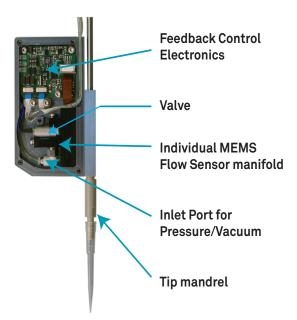
An inlet port provides aspiration/dispense pressure to the channel. A solenoid valve is coupled to a silicon MEMS flow sensor that controls the pipetted volume and allows precise tracking of the operation of the channel.
