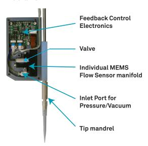
The Flow sensor and the control electronics provide precise Liquid Level Detection (LLD) on a per channel basis. The LLD signal can be read via a hardware line. Triggering of pipetting actions can be driven via a hardware line, in addition to being operable via software command on the serial line. A wide range of applications can thus be rapidly implemented.
