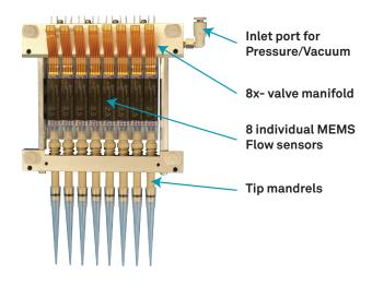
The Flow sensor and the control electronics provide precise Liquid Level Detection (LLD) on a per channel basis. The LLD signal can be read via a hardware line. Triggering of pipetting actions can be driven via a hardware line, in addition to being operable via software command on the serial line. A wide range of applications can thus be rapidely implemented.
